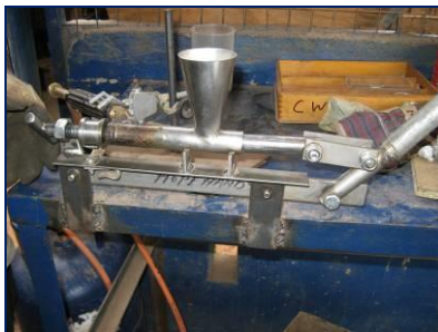
Figure 2.8 Hand extruder for washers (Senegal)
