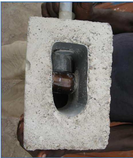
Figure 2.4 Large diameter glass bottle bearing (Ghana)
