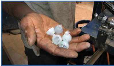
Figure 2.9 Washers produced from granules or waste plastic (Ghana)
