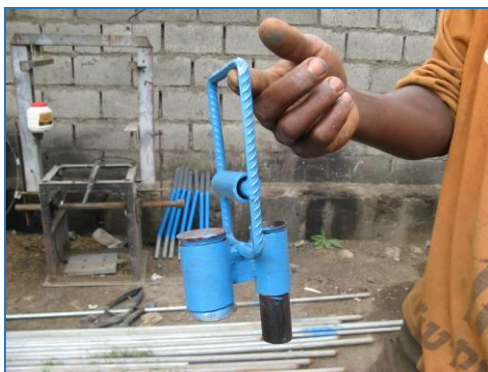
Figure 2.2 New bottom guide box, Abebe Garage Zuway
