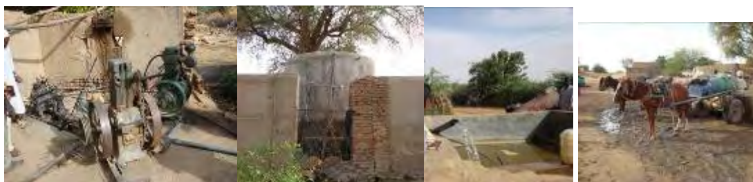
Water is pulled up by motor and pumped to storage tanks before being passed on to purchasers
