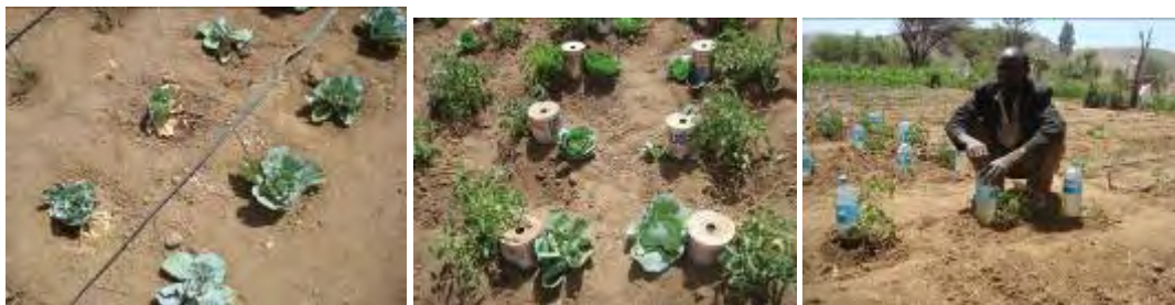
Drip technologies being tested: Imported, tin and plastic bottle (from left to right)
