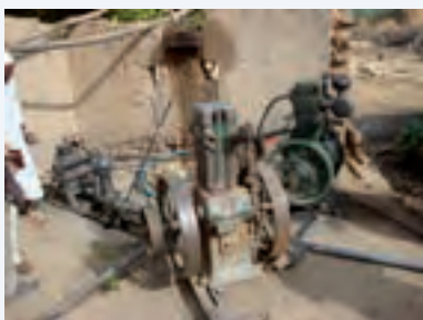
The water is pumped up from the well, to a storage tank and then fills water tanks pulled by horses.
